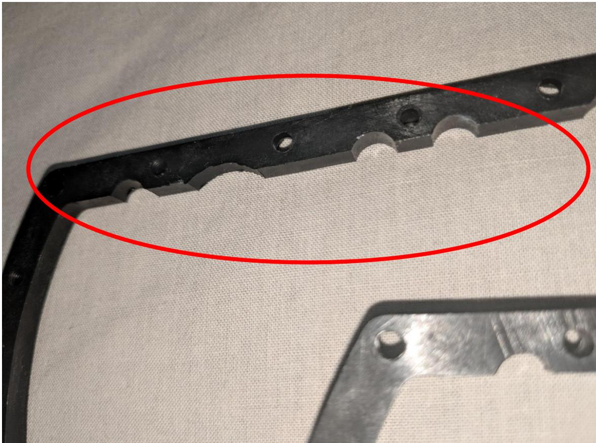
2. After most unwanted parts are remove (De Burrs) form both Mid unit. Place FEP flat on top of one of the Mid unit. Make sure all Nut slot are not facing the FEP film.
