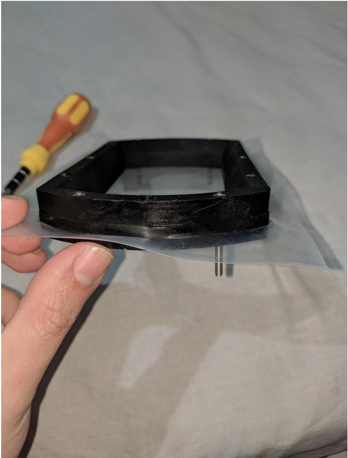
8. Now fasten rest of the 4-empty slot with “M3\*16” and M3 Nut.
