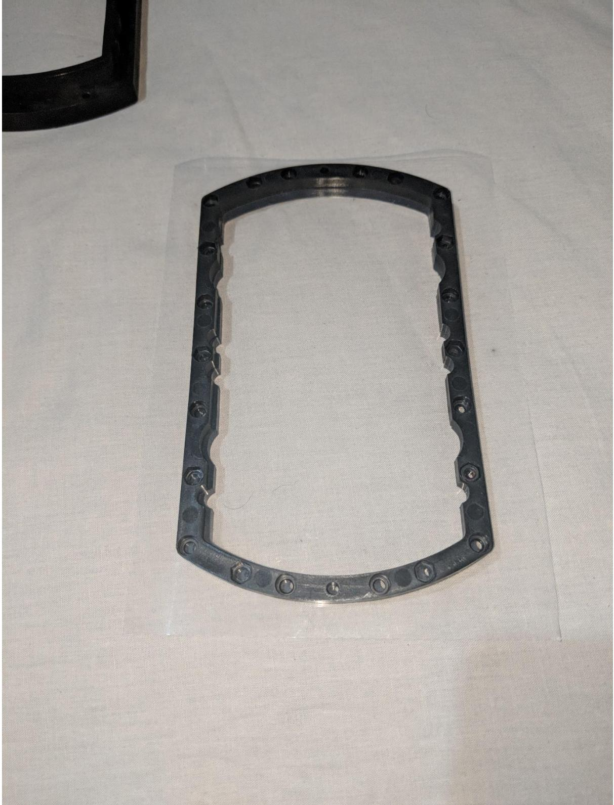
4. Aligned FEP evenly (flat will do, don't need to have slack.), Then fasten all 12 X M3\*6 with Nut on both Mid unit and FEP together with a M2.5 Hex Screwdriver. (Just poke through the Hole and ensure the whole Mid unit are evenly tighten)
