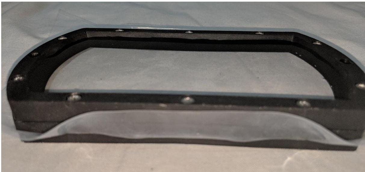
**9. Once water Leak testing are completed. You can use a Hobby knife or Pen Knife to trim of the excess FEP film. And you are done.**
